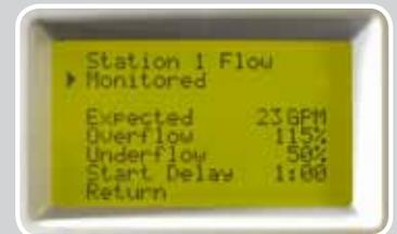
Flow monitoring capability and control at your fingertips. Flow monitoring can be programmed for each station.
